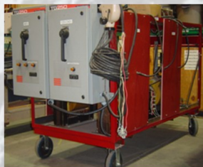
3 Phase Rated Voltage Cart Up to 14.4kV
