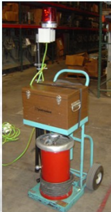
Low Frequency Withstand Test Set—100kV
